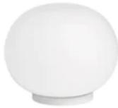
Table/desk lamp providing diffused light. Diffuser consisting of an externally acidetched, hand blown, flashed opaline glass and an injection-molded, white PBT (polybutylenterephthalate) threaded ring nut. Injection-molded, white PBT (polybutylenterephthalate) cover, base/ lamp-holder support.
